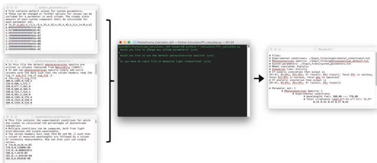
Fig. 3 Overview of computational tool. Schematic overview of the computational tool. Given the input answers to specific questions (see Subheading 2.3) the Python script simulates levels of phytochrome system components. The output is in tabular form, providing the values for each experimental condition requested
